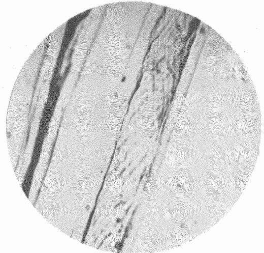
Figure 7—Part of a Cotopa Fibre. The Lattice-Like Appearance is Due to Two Sets of Spiral Markings Being Seen at the Same Time (Magnification 1000 X).
